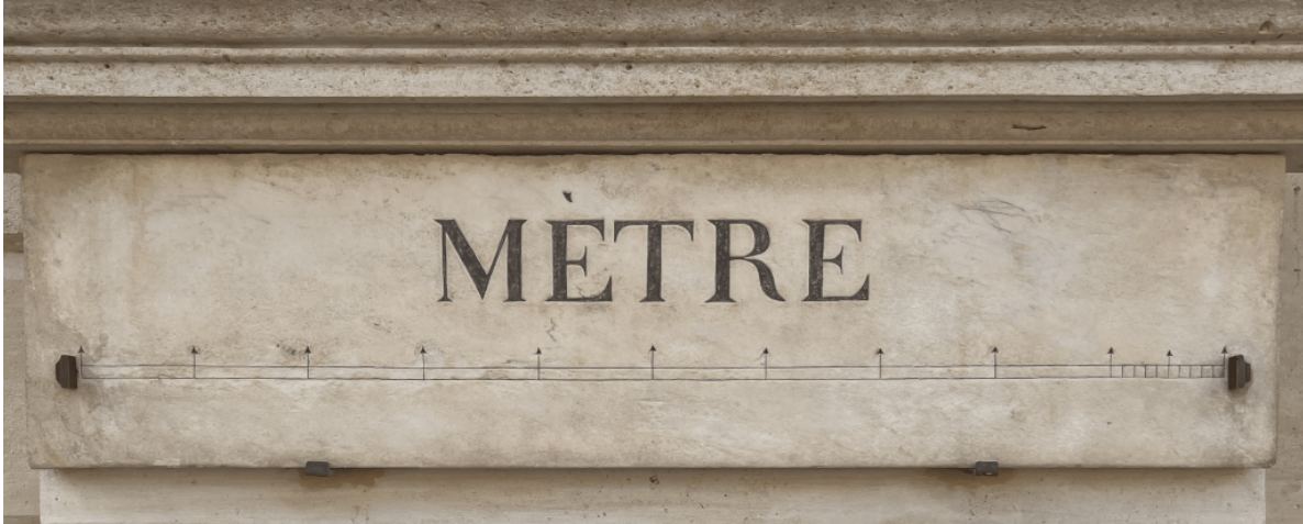
Materialization of length after the French Revolution: public meter pattern, Place Vendôme, Paris.
